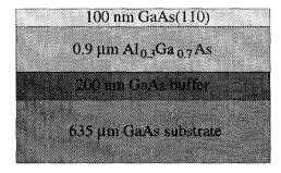
Figure 1: Schematic of standard cathode material
