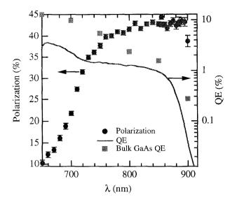
Figure 2: Polarization and QE of standard material.Bulk GaAs QE is shown for comparison. Note that in the region of highest polarization the QE of the bulk GaAs is only a factor of two greater than that of the standard material.
