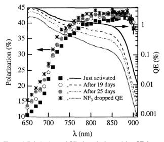
Figure 4: Polarization and QE of standard material as QE decays. The last data set was acquired by dosing the sample with  $NF_3$ . The source lifetime (e-fold time) was 26 days.
